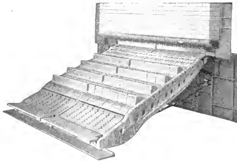
FIG. 2 INTERIOR VIEW SHOWING GRATES AND PUSHERS
